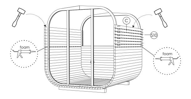
**STEP 10:** If needed, use thinner staves (H1) to fill the gap between (H) staves and apply foam between staves. Install metal bands over the screw holes, then tighten the bands.
