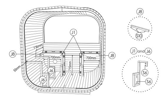
**STEP 12:** Install sauna benches on top of legs (J) using S6 screws 5x70SS. Bench cross boards have to match the tops of the bench legs. Check distances from walls, then fix benches on the legs.
