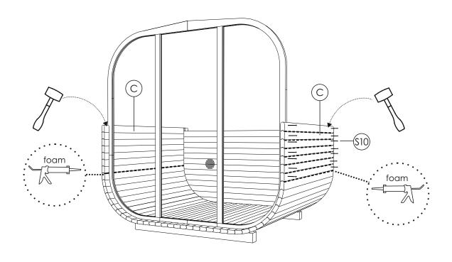
**STEP 8:** Install the panoramic panel (V1) with caution. Attach adhesive tape along the panel edge. Use foam between panels for better insulation. Place it on top of the lower back panel. Check that side edges are aligned properly with both panels. One keeps holding the panel in line, and the other is fixing the side stave on a curve using screws 4x60(S10). Check levels and fix the panel with screws at the ends of the panel's lower sides using screws 5x120(S4).
