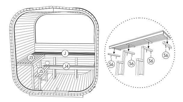
STEP13: Install the ceiling board (O) in the middle of the ceiling, pre-drill holes for screws 4x40SS (S11). Fix the backrest (J2) in front of the panorama window, first 150mm up from the sauna bench. Then install backrest staves (J7) pre-drill holes for screws 4x40SS (S11), at the same height as the backrest on the panoramic wall. Put in the flooring duckboard (L).
