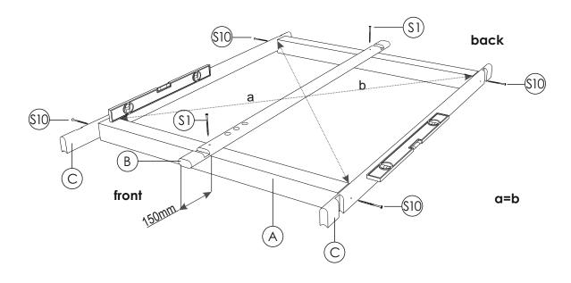
**STEP 2:** Fix 6 staves (C) to each side from the center stave. Check levels while installing staves. After 6 staves are installed, take off staves that are on both sides of the cradles and fix them next to the 6th stave on both sides. Drill 10mm hole in each staves front and back groove to the outside. Every dark point on staves is for a screw.
