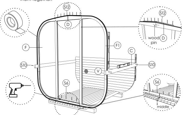
STEP 5: For both sides, the 8th to 10th stave (C) needs to be fixed as one piece. One is holding those three staves, and the other is fixing only the 10th stave with screws 4x60(S10). Between every stave use foam for better insulation.
