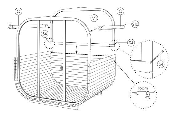
**STEP 9:** Fix the rest of the staves up to the middle of the roof. Use a rubber hammer if necessary.
