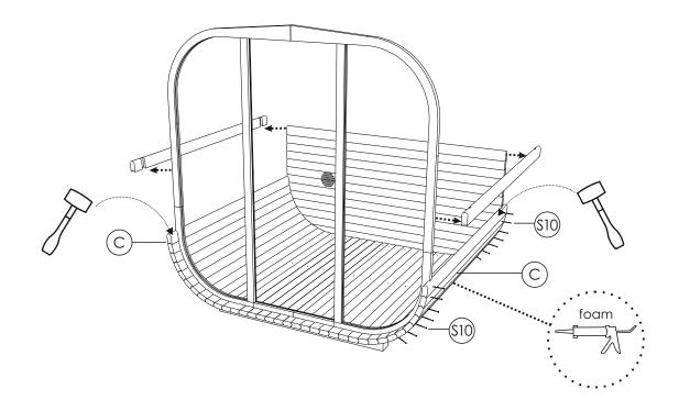
**STEP 7:**Fix the next board staves (C) on both sides with foam between the staves fix with screws 4x60(S10) for each side. Use a rubber hammer if necessary. Continue fixing staves on both sides as shown. At one side fix one board more than on other.
